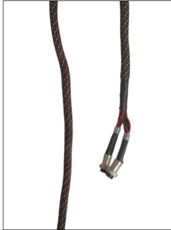
Figure 5: Removable speaker audio cable with view of the two female GX16 8-pin connectors.
