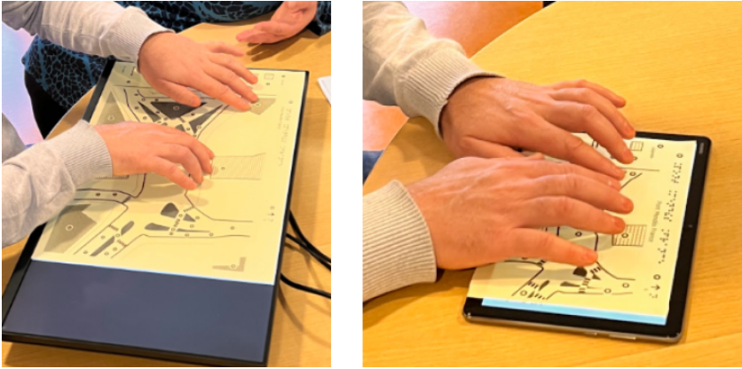
Fig. 3. P2 exploring an audio-tactile map of two different sizes: large tactile screen (A3 size) on the left and tablet (A5 size) on the right. The audio-tactile map is made of a tactile overlay placed over a touch sensitive screen or tablet. Audio descriptions are triggered when the user touches interactive zones of the tactile drawing.
