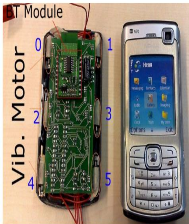
Figure 2.18 Six vibration motors integrated in a mobile phone, placed to maximize the distance between them. The motors can be controlled using a Bluetooth connection [Sahami et al., 2008].
