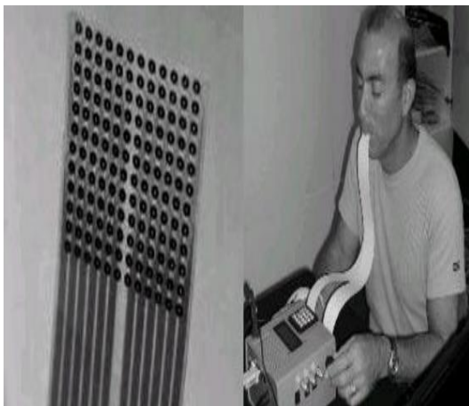
Figure 2.16 A tongue display unit (TDU) with a model of 12x12 array of electrodes [Bach-y-Rita et al., 2002] [Kaczmarek, 2011].
