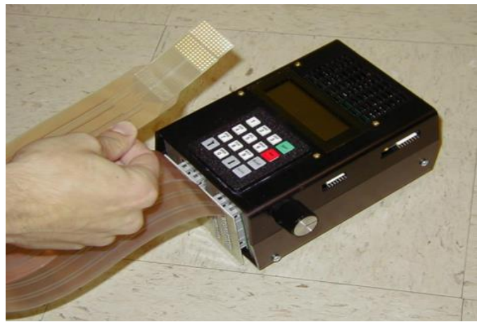
Figure 2.16 A tongue display unit (TDU) with a model of 12x12 array of electrodes [Bach-y-Rita et al., 2002] [Kaczmarek, 2011].
