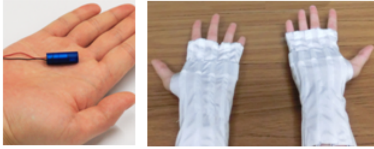
Figure 48 – Left: A vibration motor. Right: Our gloves with 10 embedded motors (5 per hand). In the tactile feedback condition, individual motors are activated to represent the classifier output.
