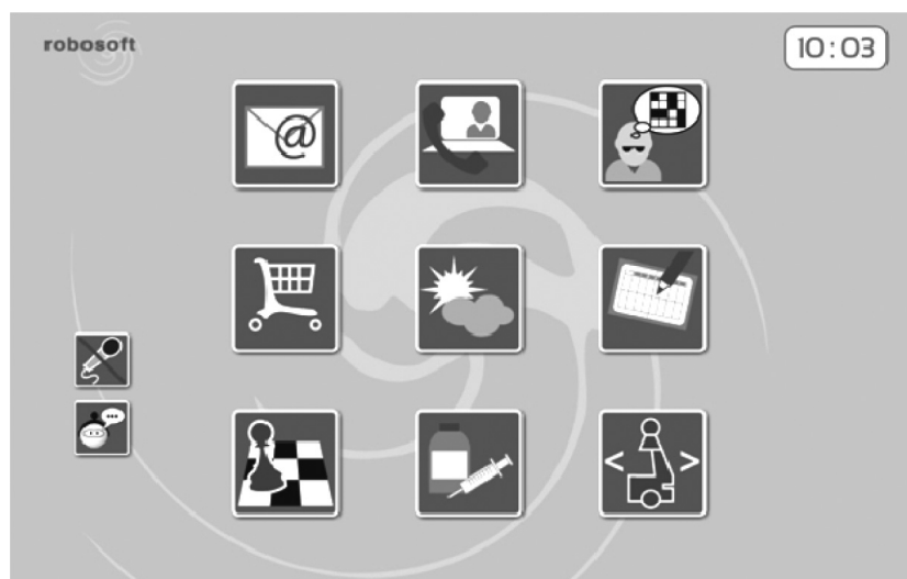
Fig. 2. Main menu screen of robot GUI. From upper left to lower right: E-mail, Video Calls, Cognitive Stimulation, Shopping List, Weather Forecast, Agenda, Web Games, Medication Reminder, and Robot Control. Smaller icons on the lower left side represent the on/of control for voice command.
