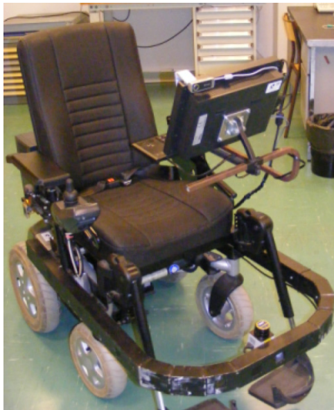
Fig. 1. Vahm-3 prototype (autonomous vehicle for people with motor disabilities).
