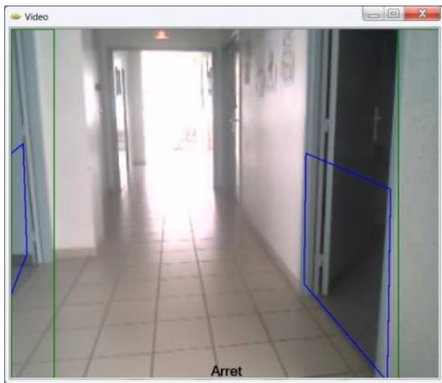
Fig. 2: Highlighted elements on the interface characterizing the features available (blue for a narrow passage, green for a wall)
