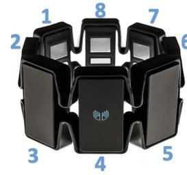
Fig. 1: MyoArmband sEMG sensors labeling.
